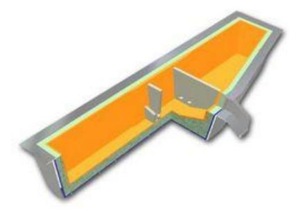
✓ Nozzles are located along its bottom to distribute liquid steel to the molds
