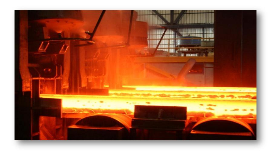
> Curved machines are used for the majority of steel casting and require bending and / or unbending of the solidifying strand.
