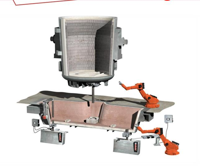
✓ The shape of the tundish is typically rectangular, but delta and "T" shapes are also common.
