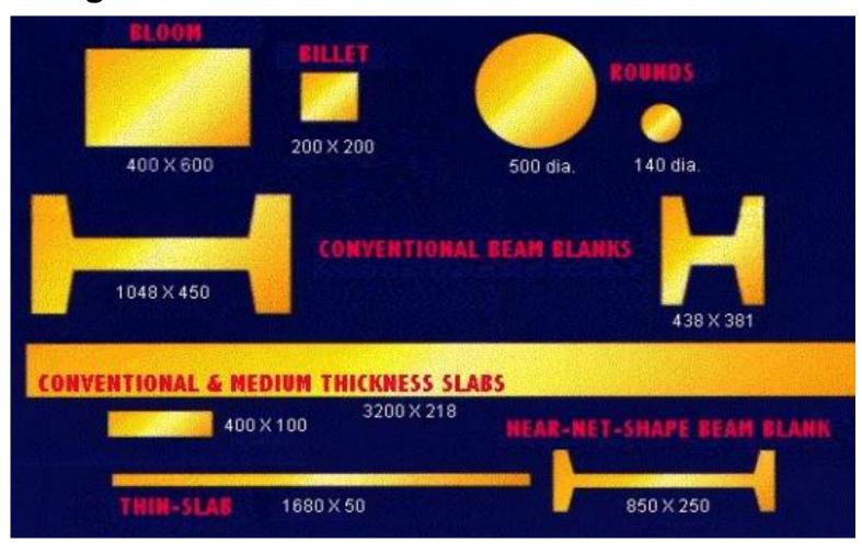
Most basic metals are mass-produced using a continuous casting process, including over 500 million tons of steel, 20 million tons of aluminum, and 1 million tons of copper, nickel, and other metals in the world each year
